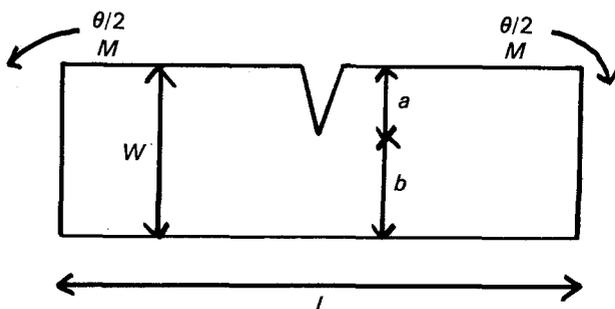
Figure 2 Model of the bend specimen configuration.
