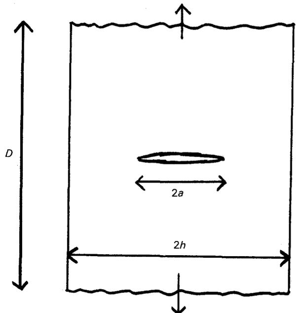
Figure 3 Model of a centre-cracked tension panel.
