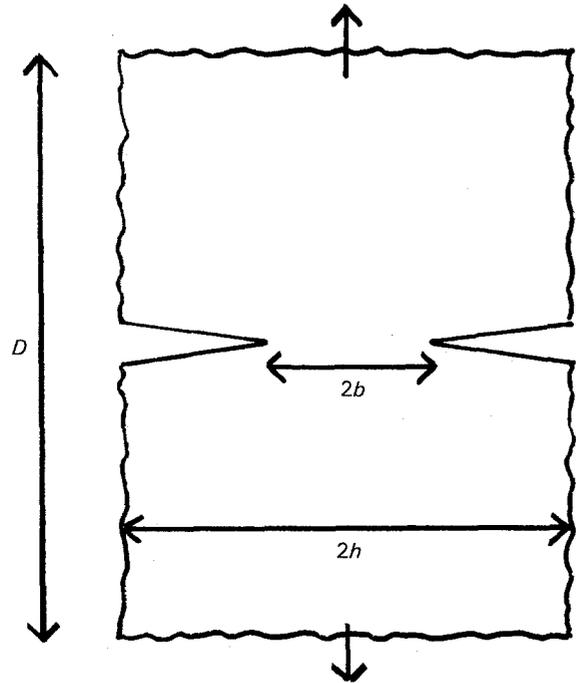
Figure 1 Model of the double edge notch tension configuration.
